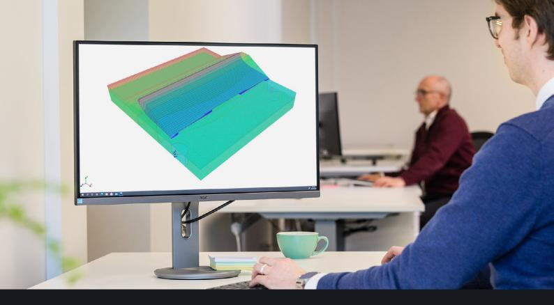
SEEP/W is a powerful finite element software product for modeling groundwater flow in porous media. SEEP/W can model simple saturated steady-state problems or sophisticated saturated / unsaturated transient analyses with atmospheric coupling at the ground surface.
