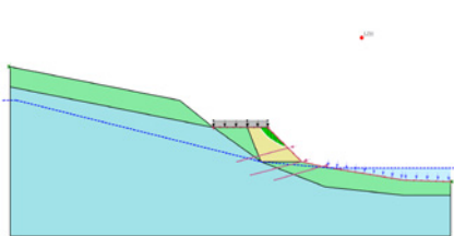
Slip surface below the road assuming weak road
