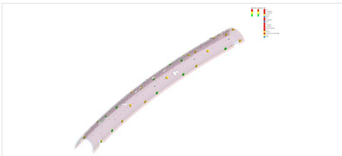
Working in an integrated digital platform reduced time for clash avoidance between structural and waterproofing and drainage collection systems by 30%.
