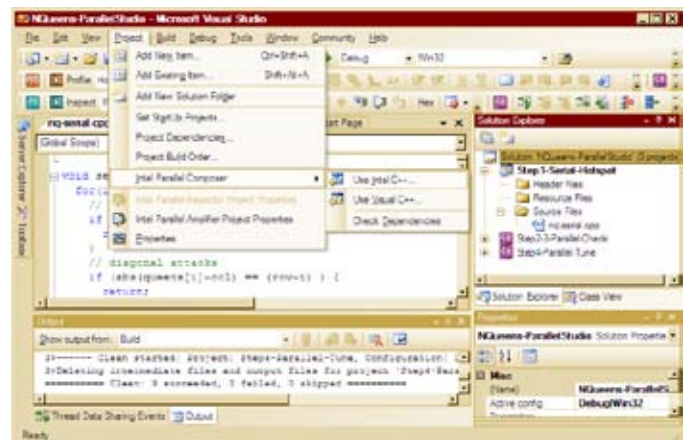
Figure 2. Intel® Parallel Composer integrates into Microsoft Visual Studio*. The solution on display shows how to switch to the Intel® C++ compiler. You can easily change to Visual C++* from the Project menu or by right-clicking over the solution or project name.
